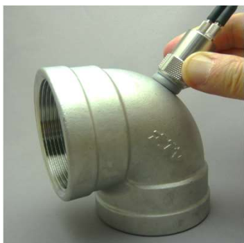
Thickness Measurement of Elbow Pipe
