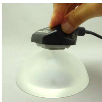
Defect Detection of Spherical Specimen (Detect Image : Triangle of flat bottom)
