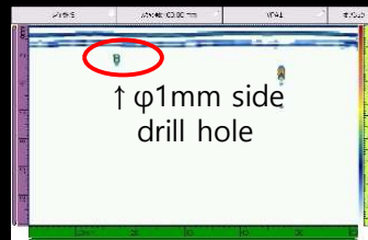
Example of a defect of φ1mm side drill hole 1.5mm surface in steel
