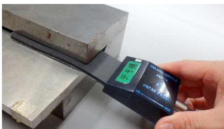
Inspection of Gaps
