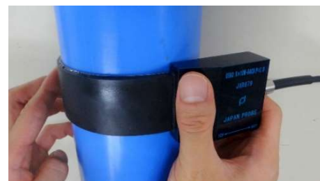
Inspection of Cylindrical pipe shapes
