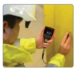
The gauges have all the features and functionality necessary to measure material thickness and velocity on virtually any material in a wide range of applications.
